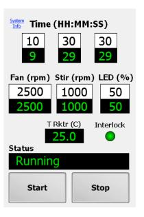
13. Once the photoredox cycle has completed, the unit will begin a 60 second post cooling cycle as indicated by the Status field. At this point the LED will stop emitting, however the fan and stir bar will continue to rotate until the countdown has reached 0.
