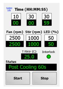
14. Upon completion, the unit will return to the stopped conditions. At this point, if necessary parameters may be changed as described in #9 and another reaction may be initiated, if desired.
