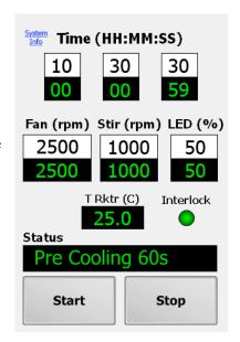
12. Once the precooling countdown reaches 0, the LED will activate at the set intensity. The Status will update to indicate that the photoredox cycle is running. At this time, the count will start from the set value and will no longer be editable. If necessary, the other fields may still be modified by changing the parameters as described in #9. Changes in set-points will take effect as soon as the "DONE" button is pressed on the dial or keypad screens.
