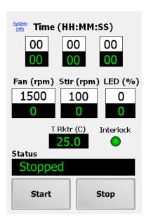
9. To change the set point of a given parameter select it on the touch screen, this will provide a display similar to the one shown on the right. The dial may be rotated to select the desired setting. Alternatively, pressing the "KEY" button will allow the user to enter an exact value using a digital keypad. Pressing the "DONE" button will accept the value.
