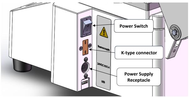
The unit must be powered with the supplied power supply (85-264V, 50/60 Hz, Full Range).
